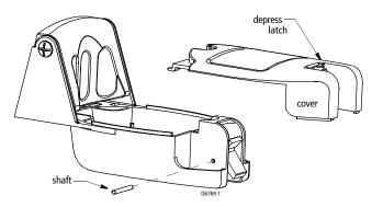
Figure 2-12: Servicing the Paddlewheel
